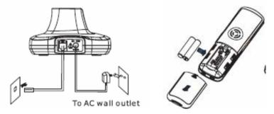
Install the rechargeable batteries in the handset. The handset requires two Nickel Metal Hydride (NiMH) AAA batteries. These are supplied with your telephone. Slide the battery cover in the direction of the arrow and pull it out. Check the battery polarity diagrams on the handset when inserting the batteries. Fit the battery cover by sliding the cover on to the back of the handset until it snaps shut.
