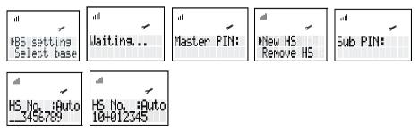
Press the **MENU** key when the unit is in standby mode.
